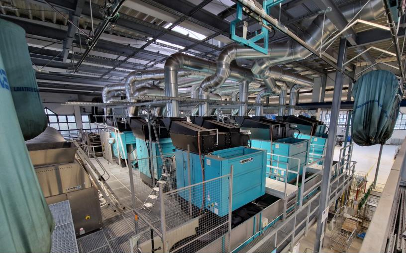
Today, after a longtime business relationship with LAVATEC, the company is enjoying the benefits of being the first in the world to install a custom built LAVACascade drying system. By significantly reducing their drying cycle, the three-tiered system with nine dryers overall has dramatically improved efficiency with a 52% gas savings and lowered associated costs.
