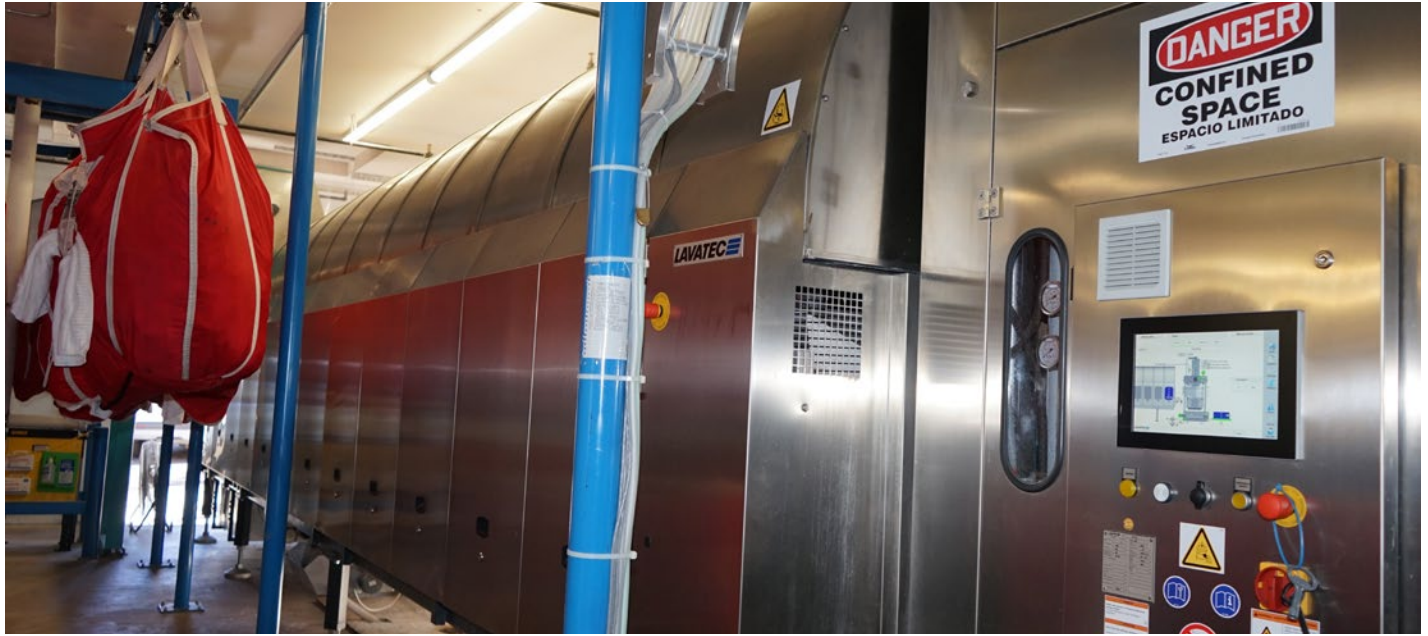
A new LAVATEC 10-compartment tunnel washer and other equipment has helped The Broadmoor's OPL produce more output while reducing operation hours, water, and energy demands this year. (Photo courtesy of TRSA)
