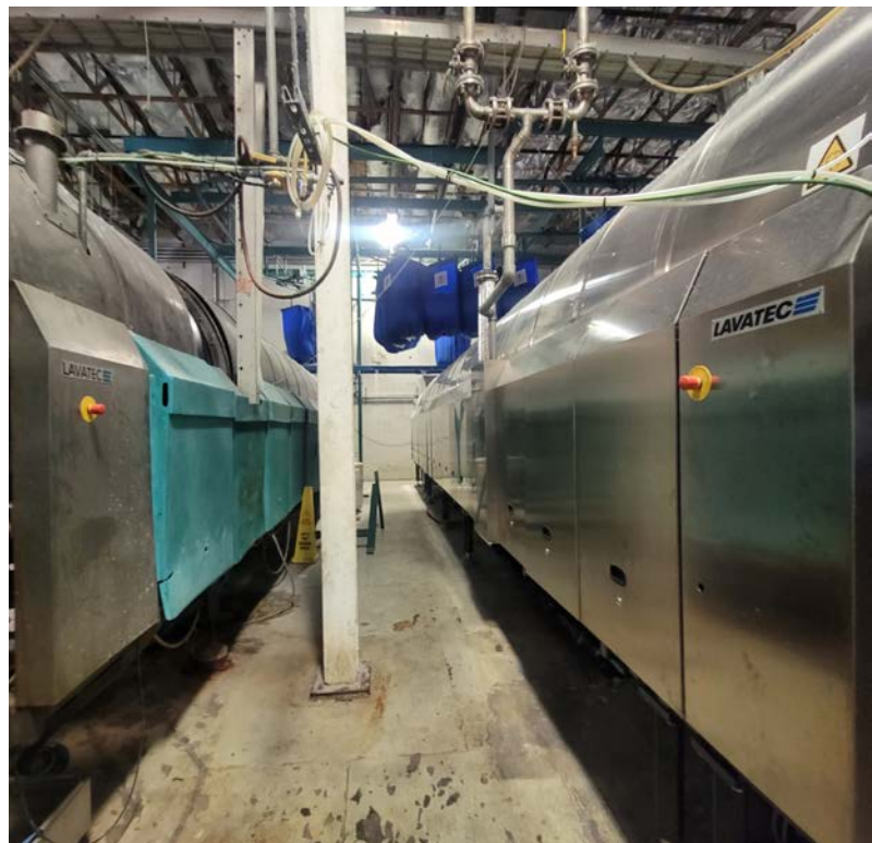
The new tunnel washer sits next to the other Lavatec that TCS has operated for over 30 years - still going strong and producing reliable results!
