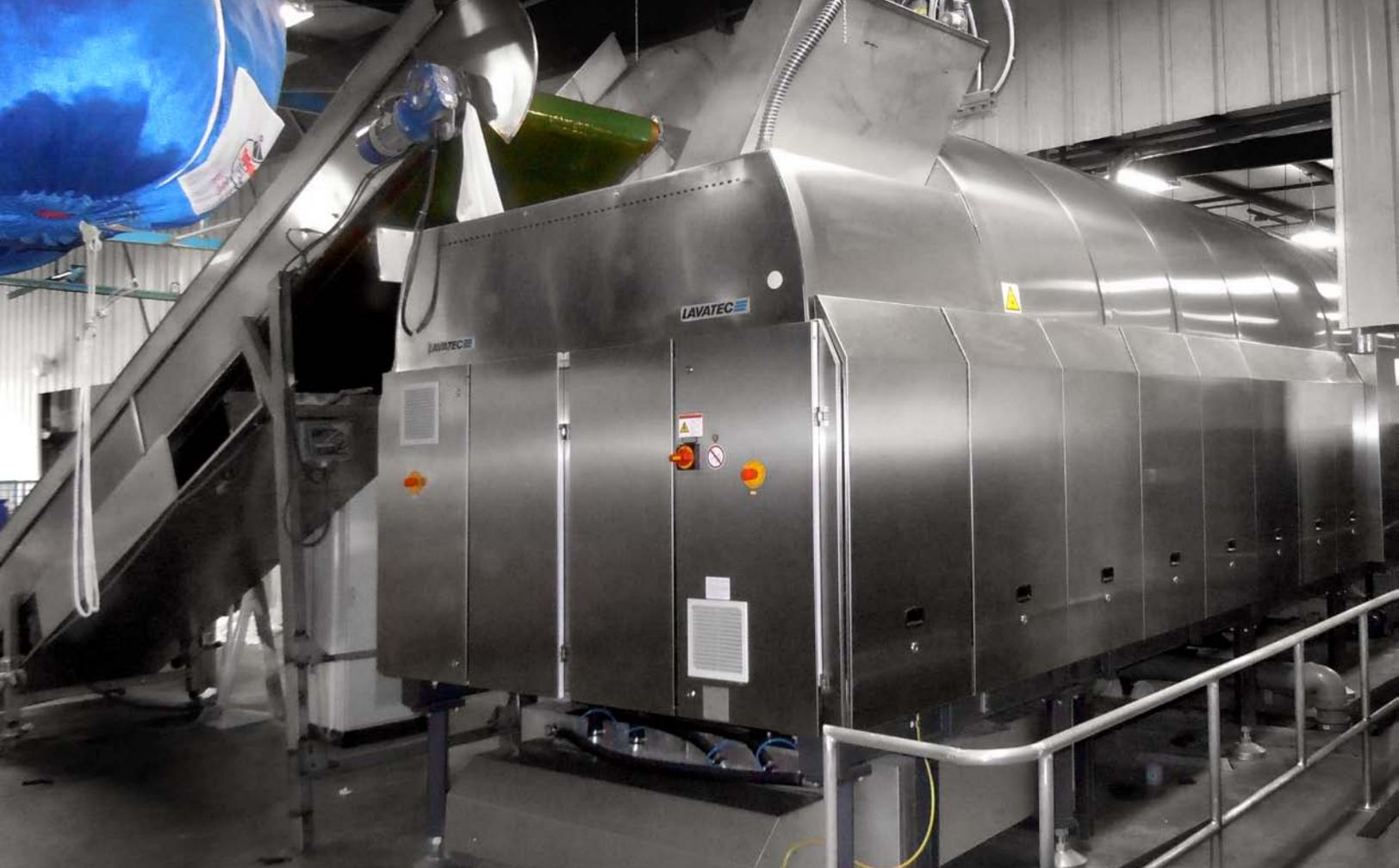
*Advantage Linen's custom new tunnel system from Lavatec Laundry Technology, Inc. includes eight chambers with center transfer, and a conveyor system that feeds two large capacity TT 745 dryers.*
