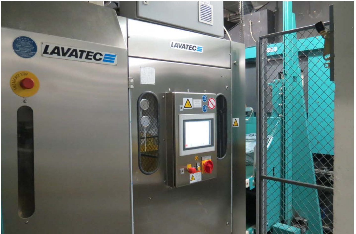
Moving up from traditional washer extractors to this 10-module Lavatec “mini” tunnel system with 25-kg (55-lb) chambers has paid off many times over since its installation at Cabell Huntington Hospital in 1994.
